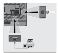
Connect the USB(HDD) USB interface on the television and the related data output on the external device (external hard disk, digital camera, card reader or MP3 player) with a USB cable;
