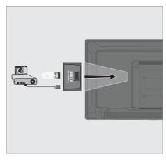
Connect the USB 2.0 interface of the television and the corresponding socket on the data device (external hard drive, digital camera, card reader or MP3 player) using a USB cable;
