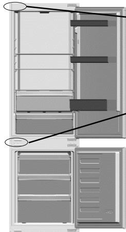
*Installation step for 10: screws must be unscrewed.*
