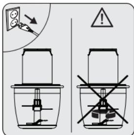
When the operation is completed, stop pressing the operation button. Unplug the appliance and wait until the blade is completely stops.
