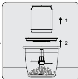
First pull and remove the motor unit (4), then the spacer lid (3).
